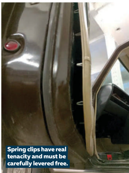
Prising off the cover of the driver's window switch.
