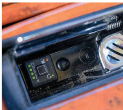
The LPG switchover button of John's Arnage is very neatly hidden away.
