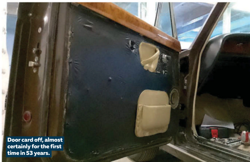
Removing the front passenger armrest bracket.
